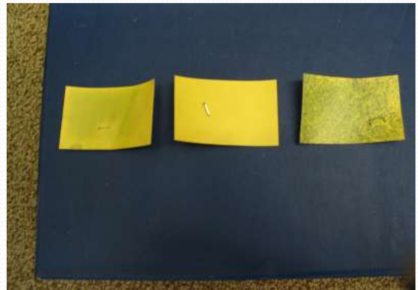
Water sensitive cards from Freeport site. Left to right: 250', 150', 50' downwind from target.
